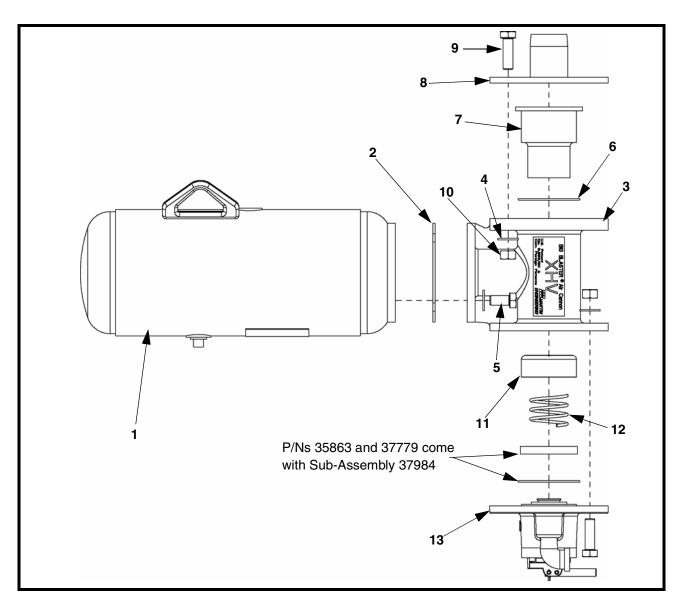
Figure 14. Martin® Tornado Air Cannon 2" Assembly, P/N 37864-XXXX\*
