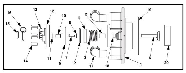
Figure 18. Martin<sup>®</sup> Tornado Air Cannon Exhaust Valve, P/N 37985
