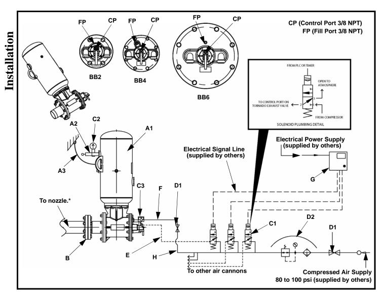
Figure 13. Plumbing Detail for Normally-Closed Solenoid Valve
