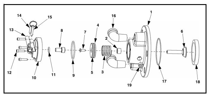
Figure 17. Martin<sup>®</sup> Tornado Air Cannon 2" Exhaust Valve Assembly, P/N 37984
