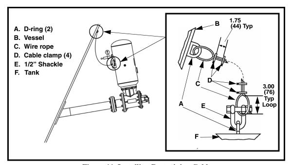
Figure 11. Installing Restraining Cable
