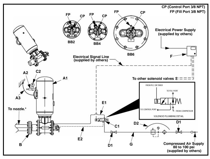
Figure 12. Plumbing Detail for Normally-Opened Solenoid Valve
