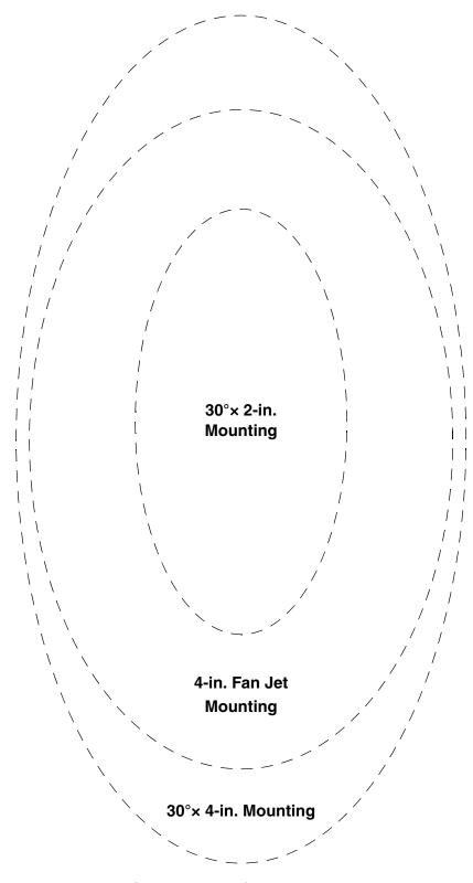
Mount 30° mounting plates vertically. Mount fan jet mounting plates either vertically or horizontally. Contact Martin Engineering for more information.
