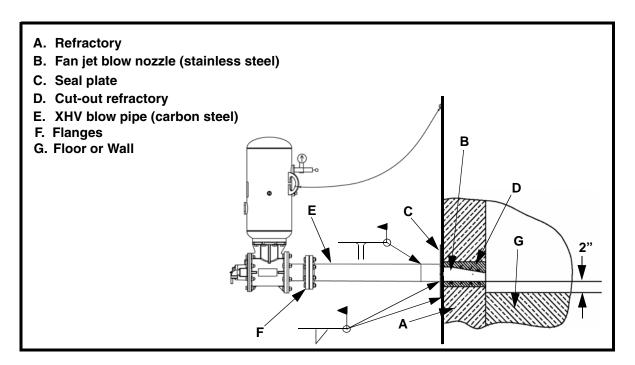
Figure 7. Installing Straight Stainless Steel Fan Nozzle and Carbon Steel Pipe for High-Temperature Applications
