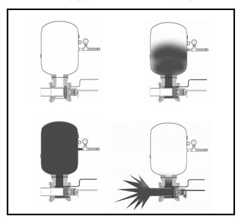
Figure 1. Air Cannon Charging and Discharging
