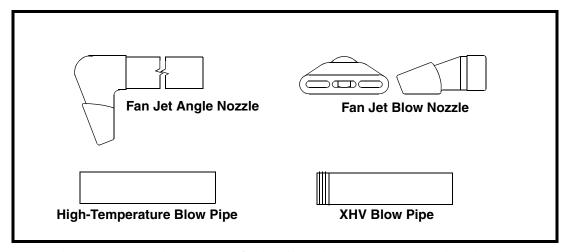
Figure 5. Mounting Nozzles/Pipes for High-Temperature Applications
