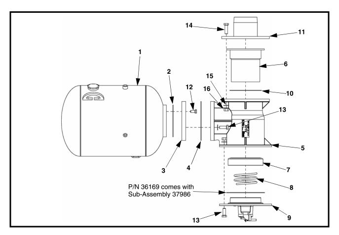
Figure 16. Martin<sup>®</sup> Tornado Air Cannon 6" Assembly, P/N 37853-XXXX\*
