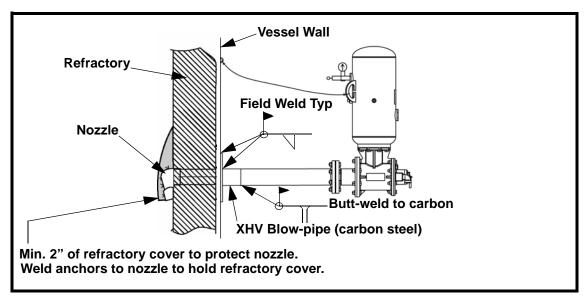
Figure 9. Installing 90-Degree Stainless Steel Nozzle for High-Temperature Applications
