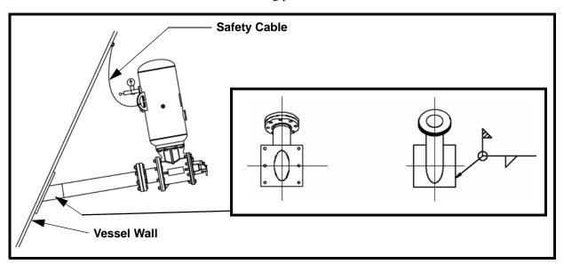
Figure 3. Installing 30-Degree Mounting Plate
