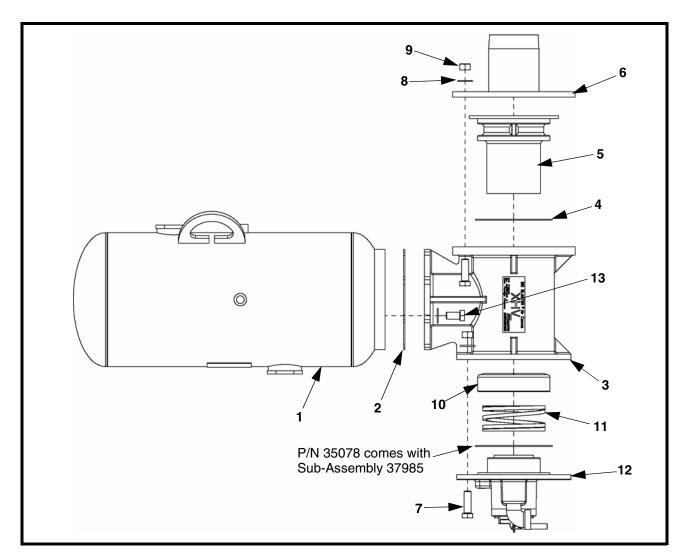
Figure 15. Martin<sup>®</sup> Tornado Air Cannon 4" Assembly, P/N 37798-XXXX\*
