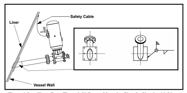
Figure 4. Installing a Drop-Through 30-Degree Mounting Plate for Vessels with Liner
