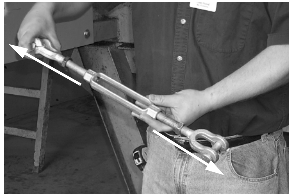
9. Fully extend turnbuckle.
