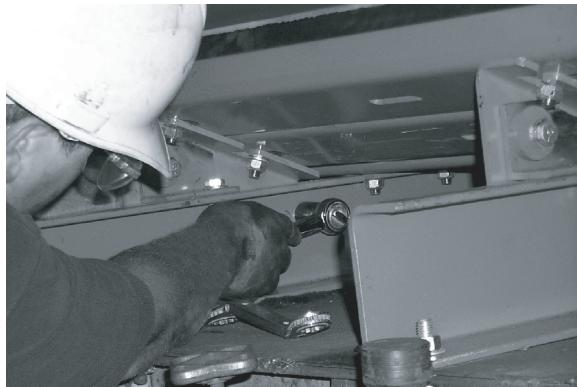
17. Rotate fine adjustment cam until wing bars are touching belt.
