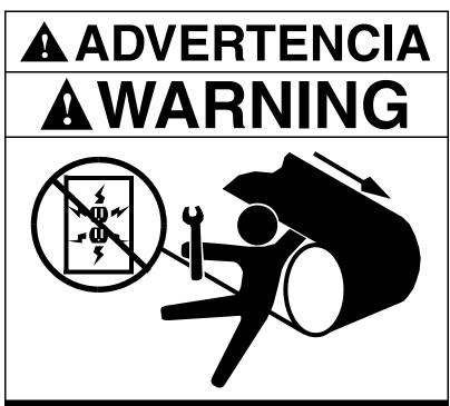
Lock out and/or tag out all energy sources to conveyor system and loading system before performing any work on conveyor or conveyor accessories. Failure to do so could result in severe injury or death.
