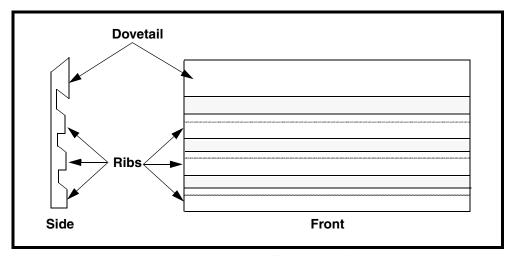
Figure 3. Urethane Secondary Seal
