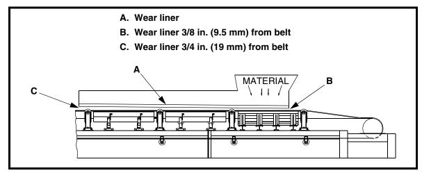
Figure 1. Locating Chute Wall and Wear Liner
