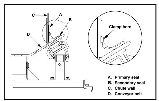
Figure 6. Installing Urethane Seals
