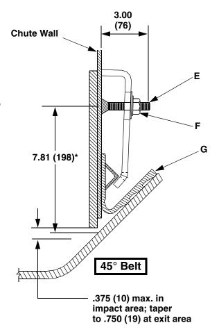
\*Distance from center of mounting stud to point on belt below chute wall.
