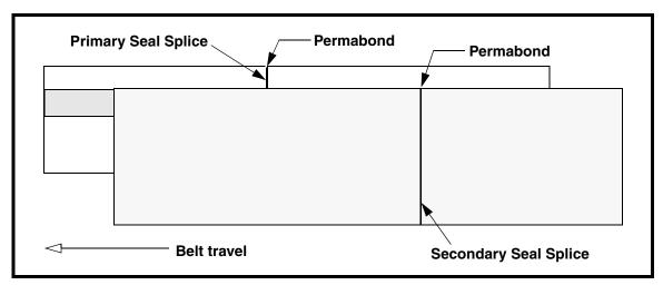
Figure 5. Staggering Splices
