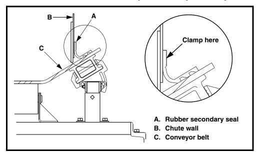
Figure 7. Installing Rubber Secondary Seal
