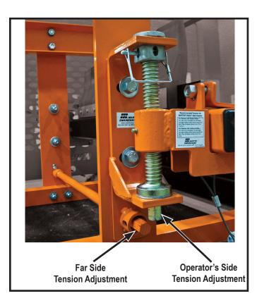
The Martin<sup>®</sup> SQC2S<sup>™</sup> Cleaner STS<sup>™</sup> incorporates individually-cushioned tungsten carbide blades for effective cleaning without risk to belt, splice, or blade. Installed in the secondary cleaner position, the Martin<sup>®</sup> SQC2S<sup>™</sup> Cleaner's blade buffers cushion impact and maintains cleaning pressure. This cleaner's extended cartridge allows the blade cartridge to be serviced without confined space entry or breaking the safety plane.
