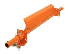
The Martin® QC1™ Cleaner PD provides maximum durability and performance across a wide range of duties and applications. This sturdy cleaner features one-pin blade change, making replacement of a worn blade a simple procedure. The one-piece urethane blade has a "CARP" (Constant Angle Radial Pressure) design to maintain cleaning performance through all stages of blade life.
