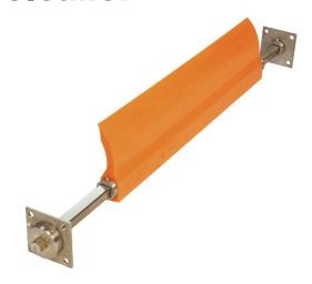
The Martin® Compact Cleaner from Martin Engineering uses a low-profile blade mounted on an internal square mainframe for effective belt cleaning in tight spaces. It is designed for applications on small pulleys and belts operating at speeds up to 350 fpm (1.78 m/sec).
