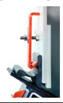
Martin<sup>®</sup> ApronSeal<sup>™</sup> Single Skirting is a dual sealing system that prevents spillage without requiring service to maintain an effective seal. Martin<sup>®</sup> ApronSeal<sup>™</sup> Skirting Systems provide dual-sealing surfaces. The primary seal is clamped to the chute wall with the self-adjusting secondary laying outward to create an effective dust seal that is out of the material flow.
