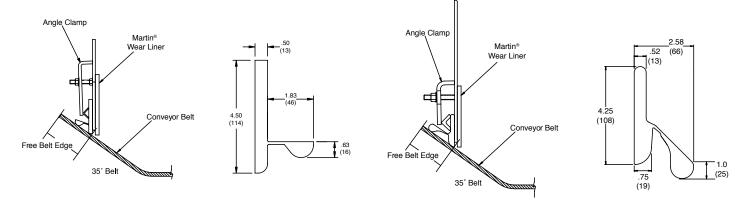
\* Martin<sup>®</sup> ApronSeal<sup>™</sup> Single Skirting is also available in food grade thermoplastic rubber and in a high-temperature silicone based rubber ordered in a 24-foot length (100724-F).
