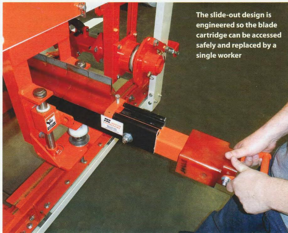
The slide-out design is engineered so the blade cartridge can be accessed safely and replaced by a single worker
