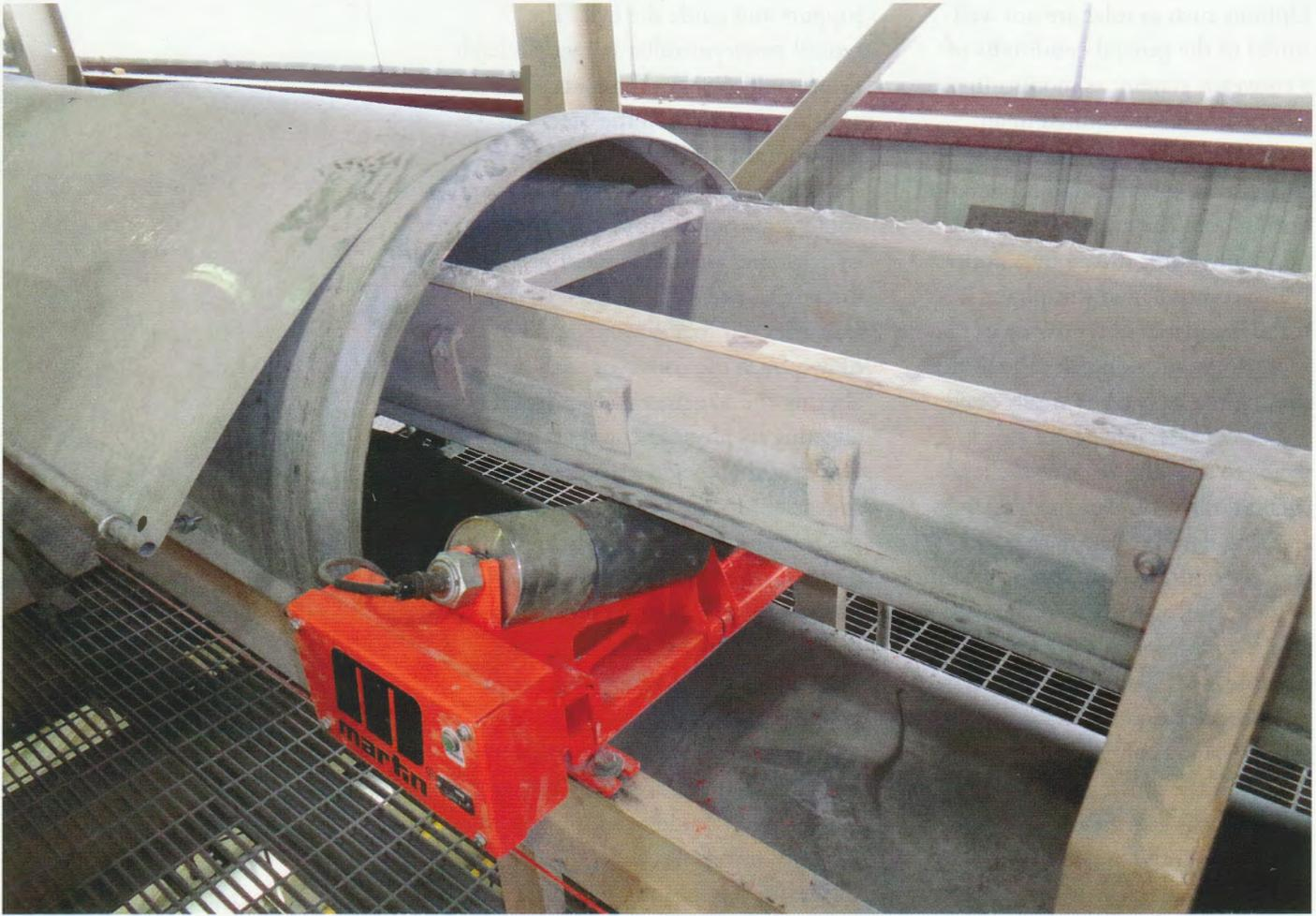
magnetic coupling that attaches to the end of an existing roller. The outside diameter of the generator matches the diameter of the roll, but places the generator outside the normal belt line to avoid the heavy loads and fugitive material that tends to damage existing design attempts. The generator is held in a fixed position by the roll support system, but is not normally required to bear any of the material load.
