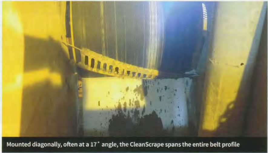
Previously the blade became encrusted with material, degrading performance and causing build-up accumulation
