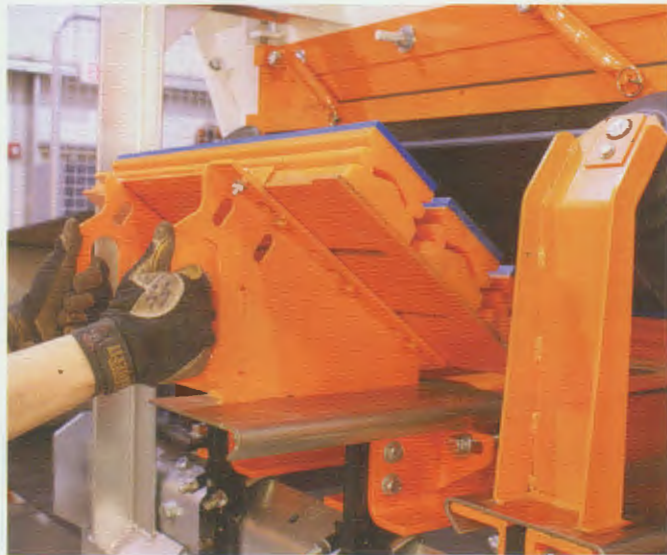
The modular impact cradle absorbs the impact of the falling load, yet slides in and out for easy service.
