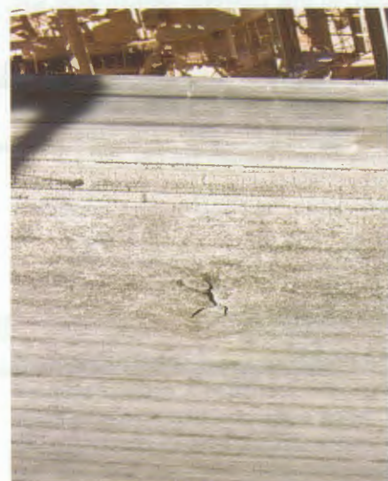
A receiving belt can experience severe damage from material transfers if it's not supported properly.
