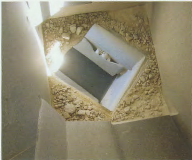
A rock box acts like a shelf, catching and distributing falling material onto the impact cradle.
