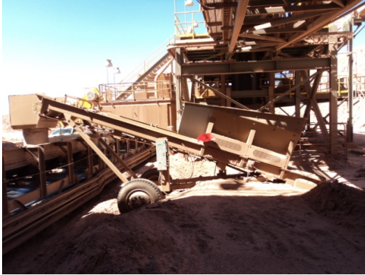
The plant was having a hard time keeping dust and fines from escaping the transfer point.
