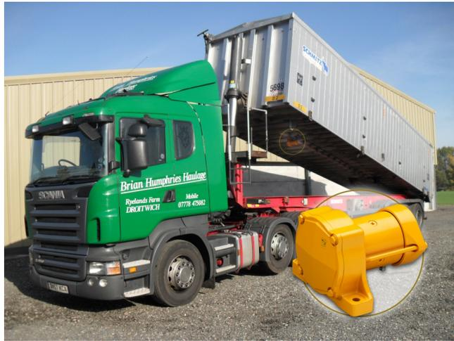
*Humphries Haulage is cutting its tipping time in half by using a high-performance 24V truck vibrator to more efficiently empty dump beds.*
