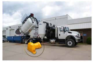
Vactor Manufacturing, one of the world's leading manufacturers of industrial vacuum loaders, hydro excavator and sewer cleaners, is employing engineered vibration technology to improve off-loading of industrial waste, including difficult materials such as dry bulk powders, slurries and even thick sludge.
