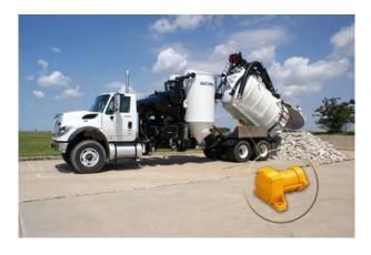
Although Vactor uses four different vibrator models for various applications in its vacuum loaders and hydro excavators, all are Cougar® vibrators. Each industrial truck gets a mounting plate, whether ordered with a vibrator or not, so a retrofit is an easy bolt-on installation
