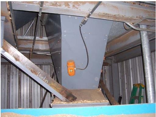
*A field-fabricated drop chute was fitted with a Martin Vibrator to eliminate plugging and improve material flow to the new transfer point.*
