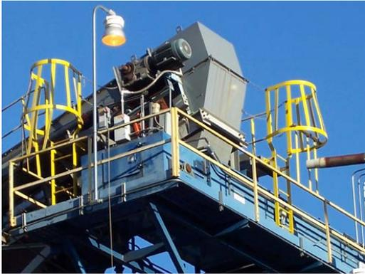
*This section of existing air-supported conveyor was modified to relieve spillage.*
