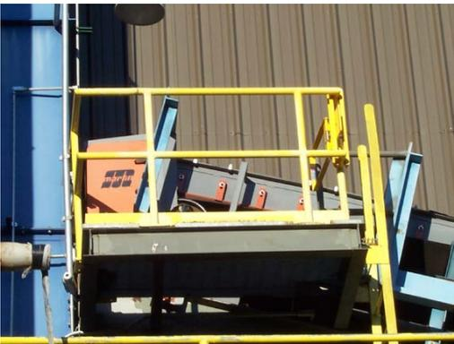
*A new head chute and brush cleaner were installed at the bucket elevator, eliminating plugging and reducing dust by an estimated 95% in this area.*
