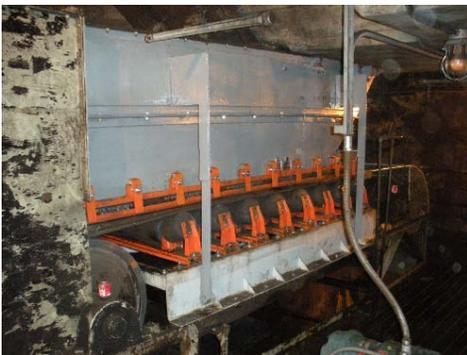
*With the EVO® External Wear Liner installed, the plant can provide effective sealing of the belt edge with Martin® ApronSeal™ Skirting.*
