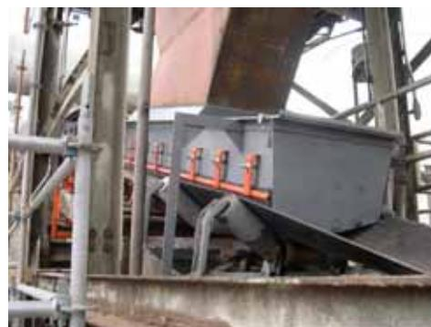
*A Martin® Tail Sealing Box was field-fabricated on each of the bark conveyors at Weyerhaeuser Pine Hill.*
