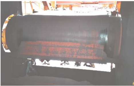
The life cycle of the blades for the Martin® DT1 Cleaner XHD has been roughly 3 years per set.
