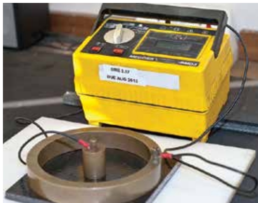
Figure 15.7. Static discharge test.
