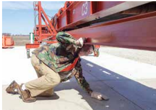
Figure 28.10. Crossing under a conveyor is a risky behavior that can lead to injury.
