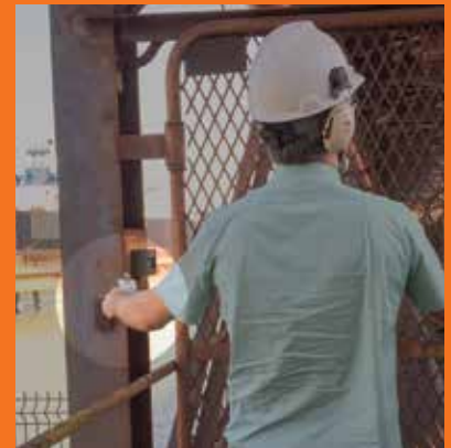
A worker uses the RFID tag on his ID card to gain access to a conveyor.
