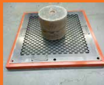
Figure 2. Test method for concentrated load on flattened expanded metal panel.
