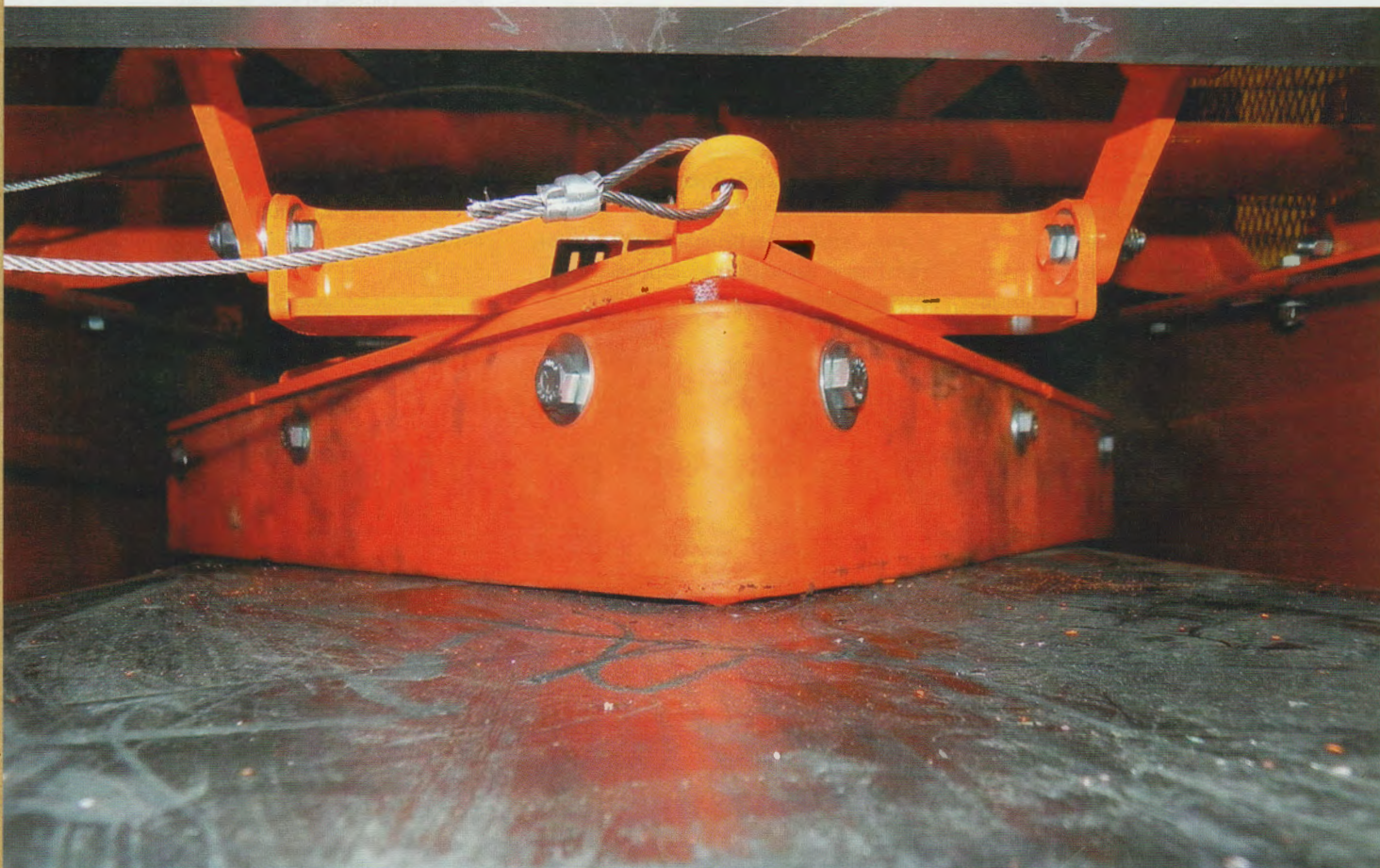
1 The V-Plow HD hub mounts can be welded or bolted to the hanger bars
