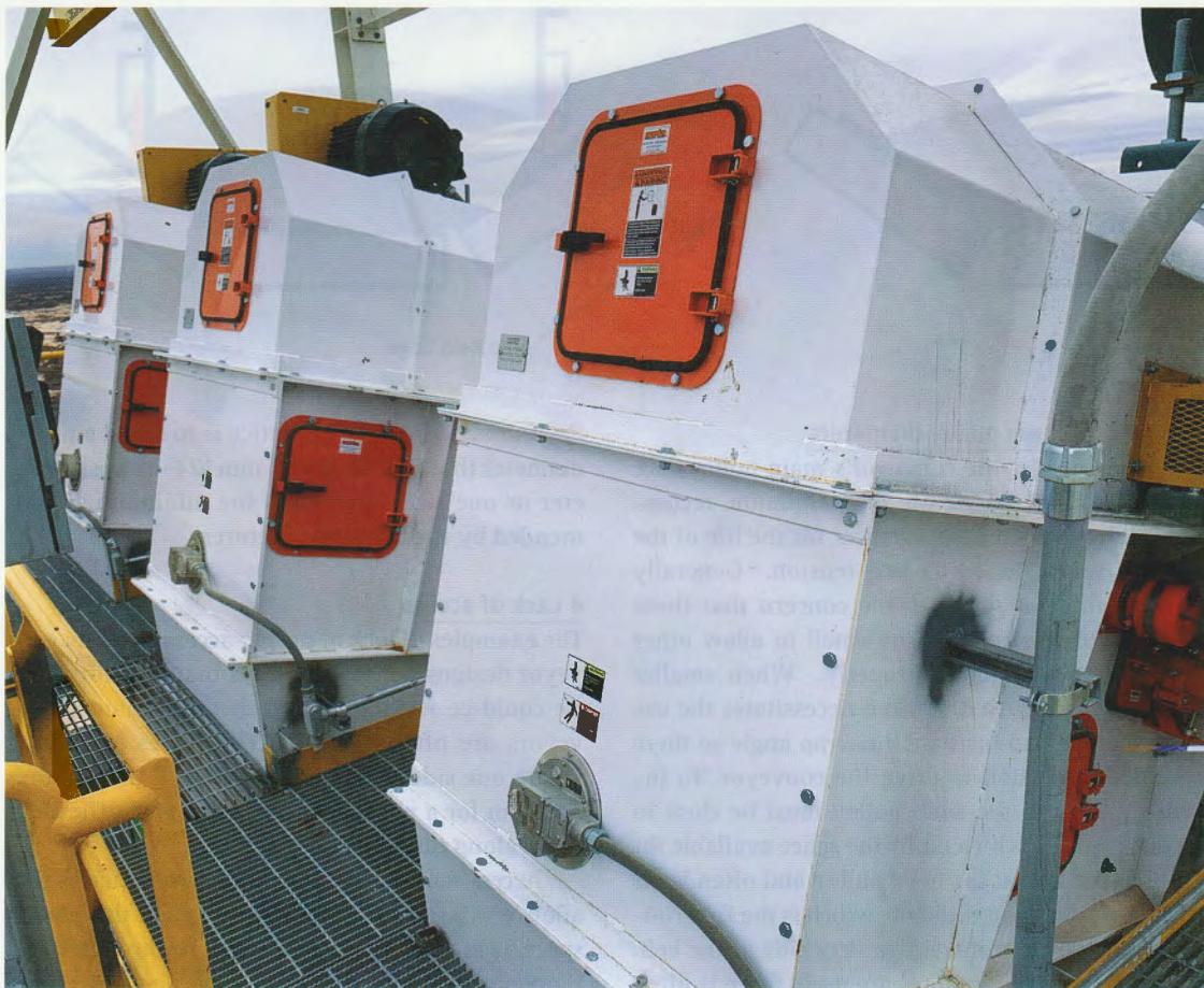
4 Strategically-located access doors facilitate inspection and service
