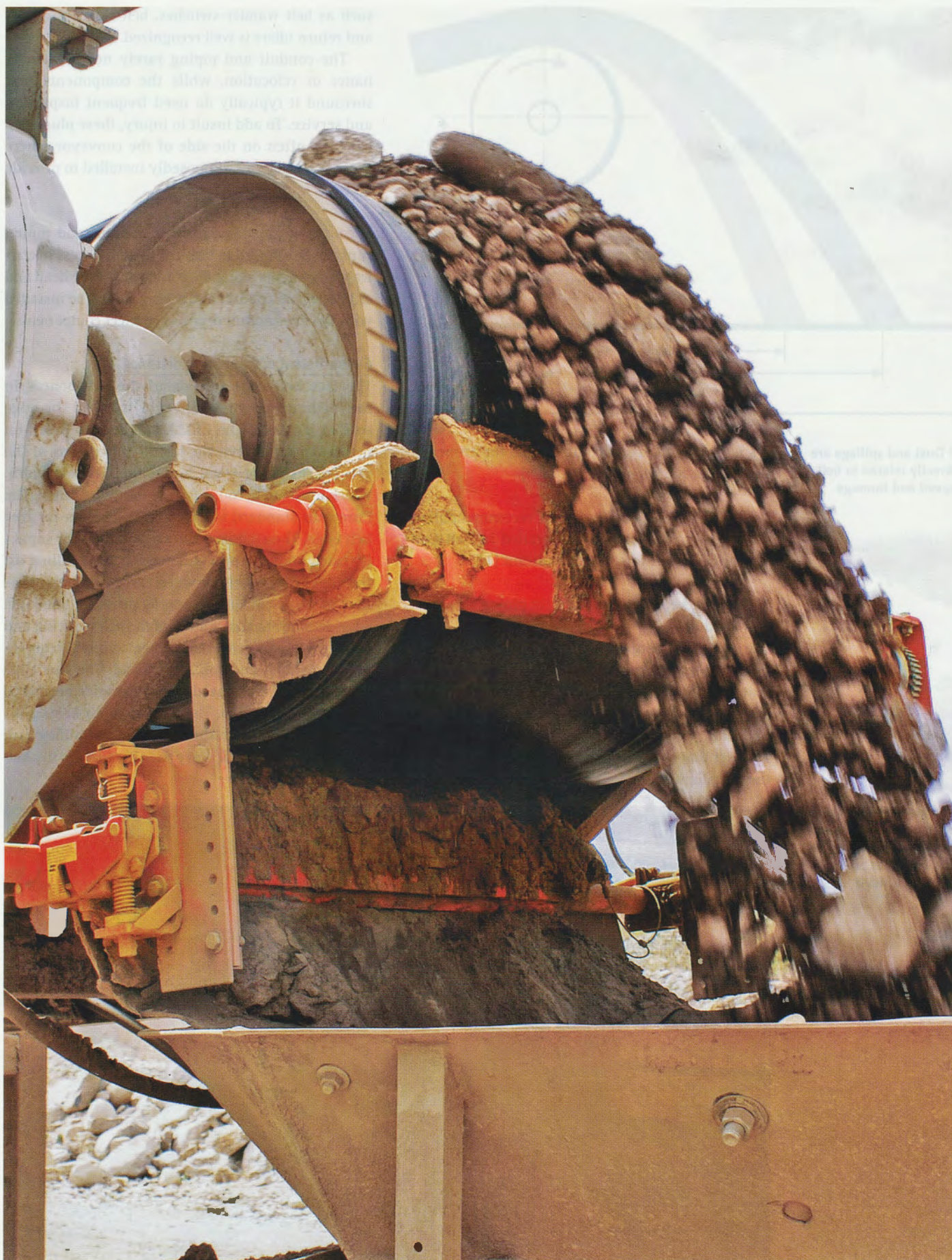
8 Adequate space and access for multiple cleaners is critical in preventing carryback and controlling fugitive material
