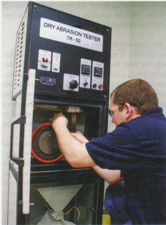
2 A dry abrasion tester checks three-body abrasive wear, such as between a conveyor belt, chute liner and bulk material
