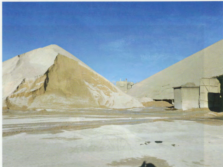
3 Limestone and other raw material is taken from trucks and barges, and stored in outdoor piles
