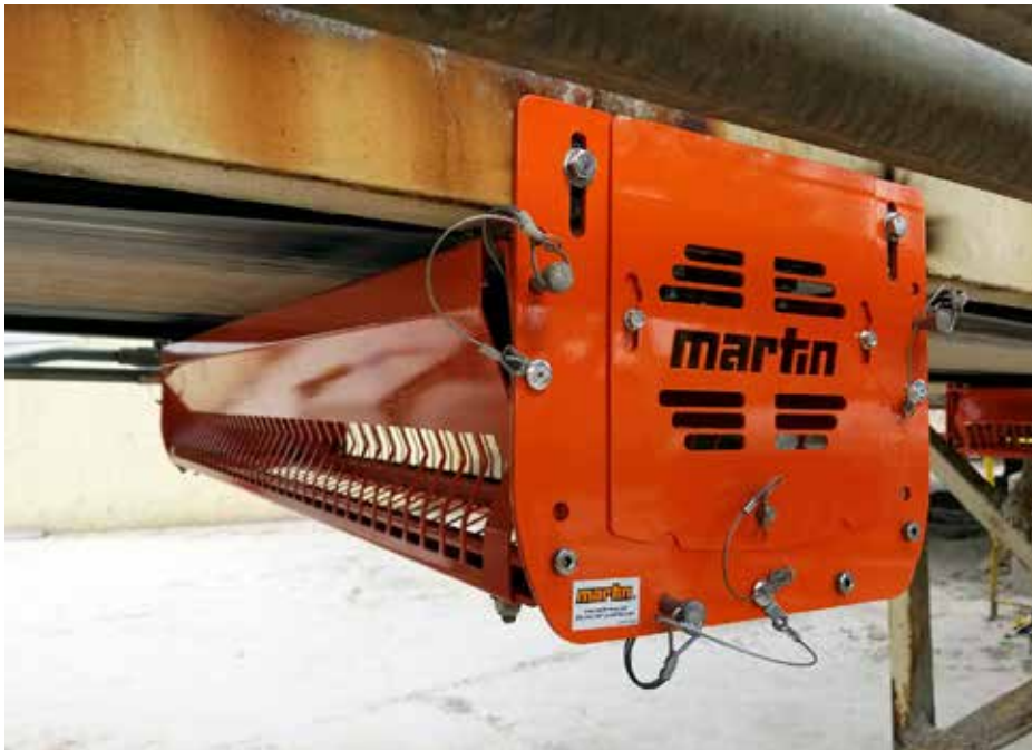
4 Return roller guards ensure detached rollers don't pose a hazard to workers or harm the system
