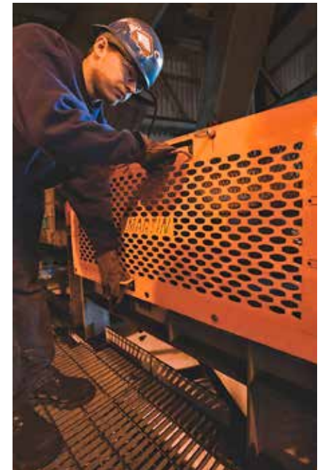
5 All moving or rotating components should be guarded, regardless of location
