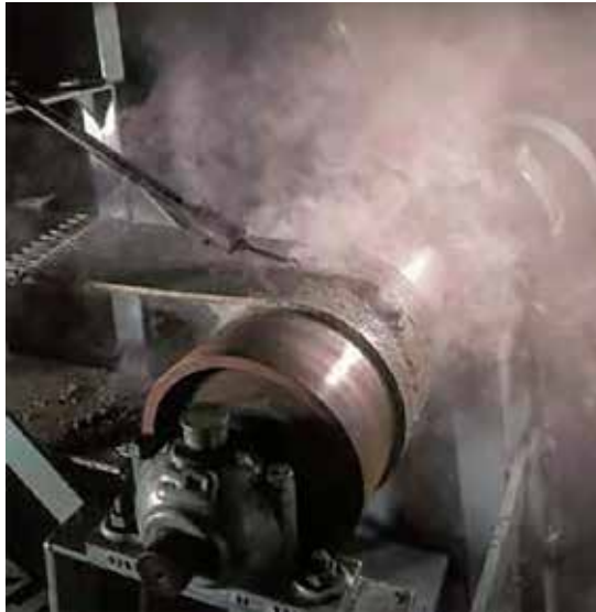
4 Friction heat between rolling components can be extreme enough to light both the material and belt
