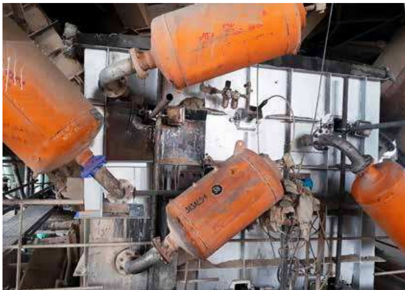
3 The old 150 l cannons with fixed pipe assemblies at Chittor Cement
