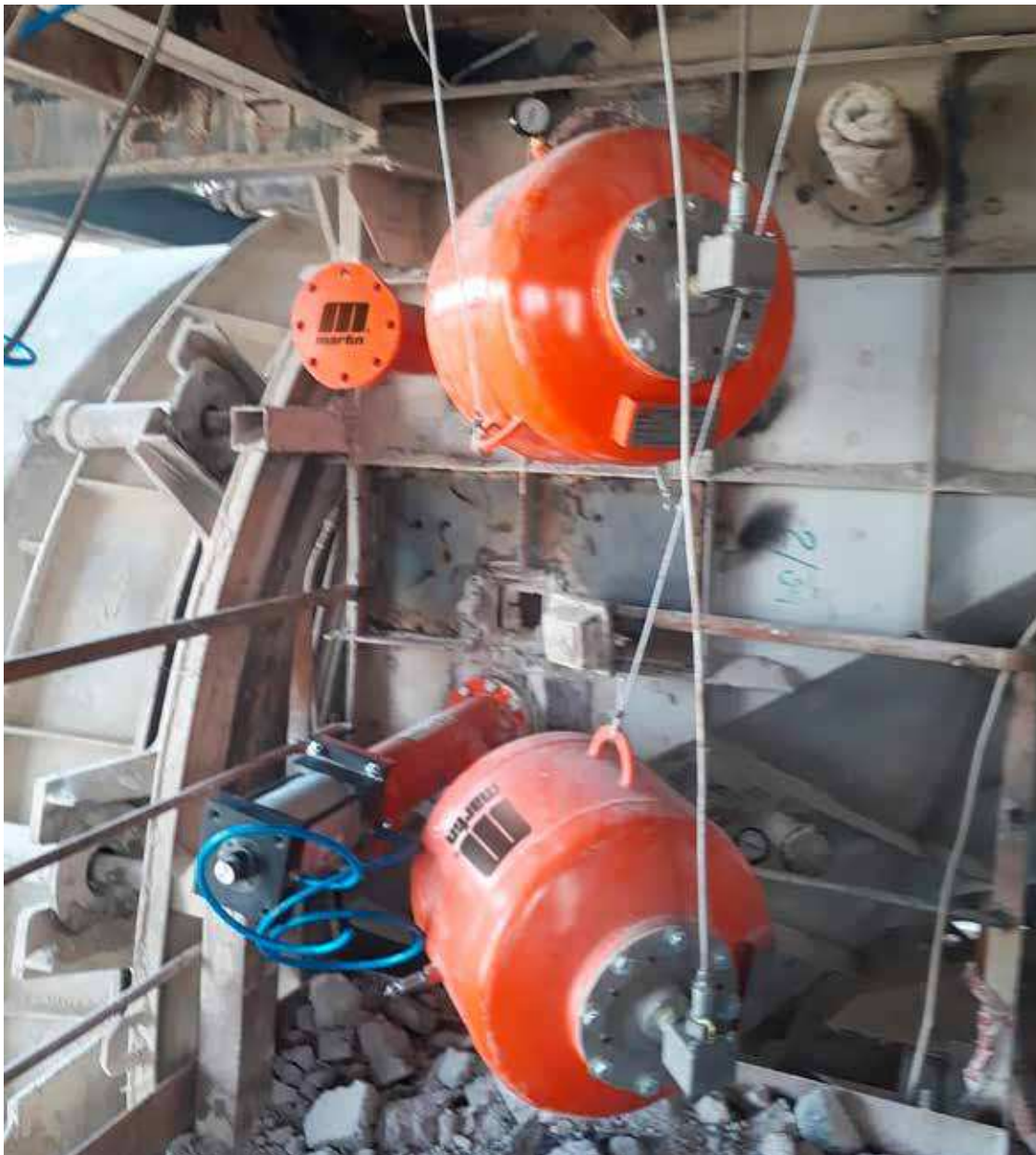
4 Two 70 l cannons on Y-pipe assemblies, the bottom one fitted with retractable nozzle
