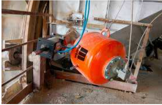
5 A single cannon to address a clog point, with a retractable nozzle to extend the equipment life
