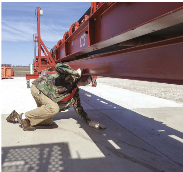
Figure 3. Taking a shortcut by crossing over or under a conveyor can lead to injury.
