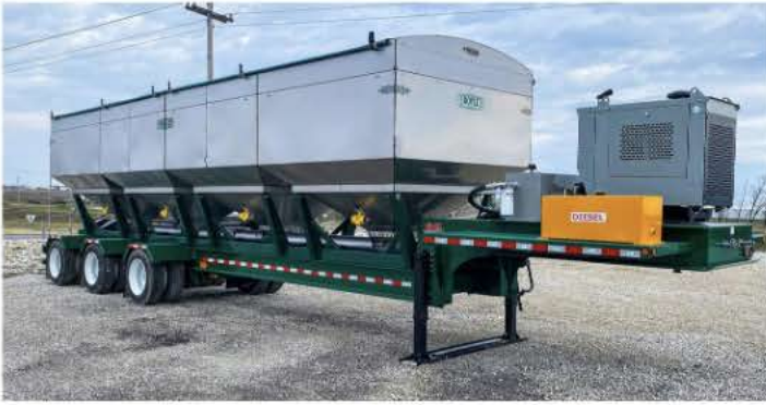
Figure 1. Doyle's 24 ft trailer tender has a modular design that allows it to be customised to meet customer needs. Copyright©Doyle Equipment Manufacturing Co 2023.
