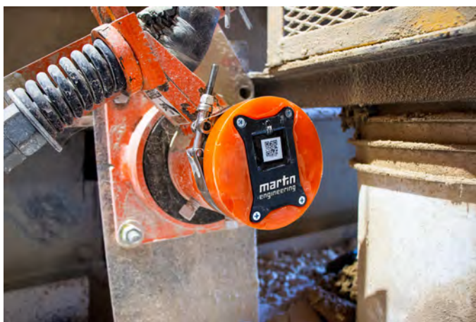
Figure 4. Blade wear indicator with remote monitoring.
