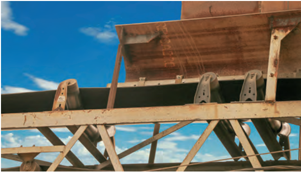
Figure 1. This is an example of a fabricated curved skirtboard, which is hard to maintain when replacing wear liners and skirting.
