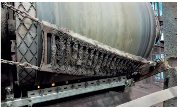
Figure 3. Offering edge-to-edge coverage, new cleaner designs are more resilient in punishing environments.
