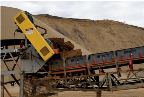
Figure 1. Impact cradles and support cradles are linked by transition rollers to avoid belt sag and retain the seal.
