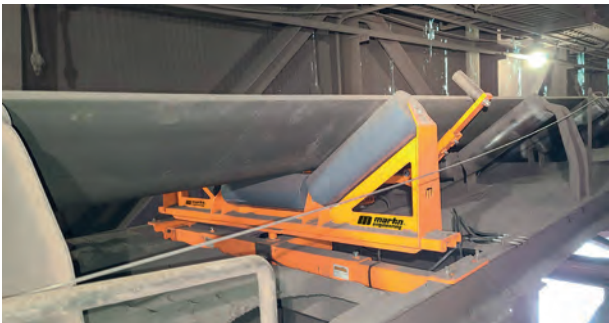
Figure 2. The tracker reacts the moment the belt drifts to make slight adjustments.
