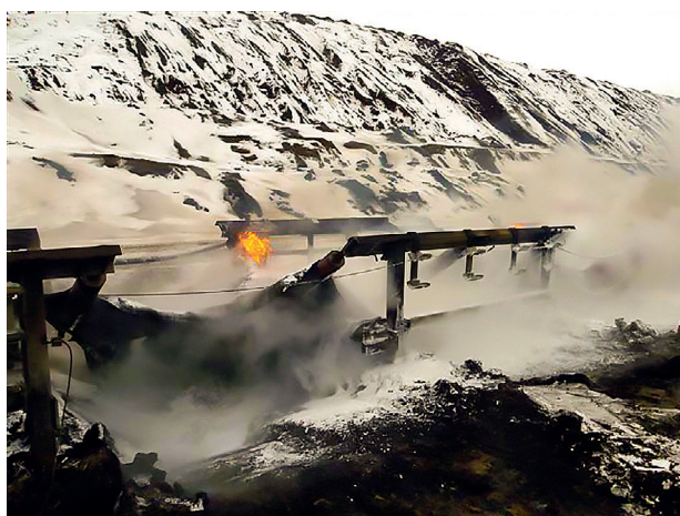
Figure 6. Coal carryback accumulation causes bearing failure, which can lead to a belt fire.
