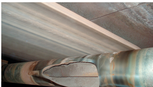
Figure 5. Damaged idler roll shell because bearings failed from fugitive materials penetrating the bearing seal.
