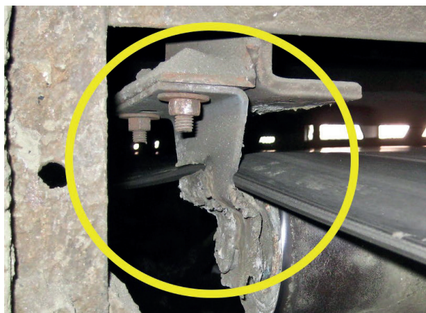
Figure 4. Buildup causes belt mistracking, which leads to belt and structural damage and a potential safety incident.
