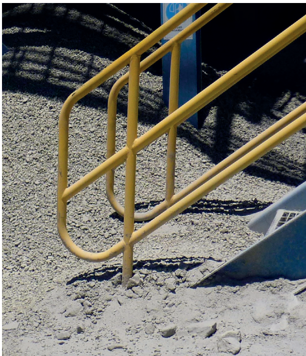
Figure 1. Spillage from transfer point causing slip, trip, and fall hazard.
