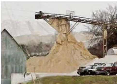
Figure 2. Sand spillage reaching up to the discharge point on a stacker conveyor.
