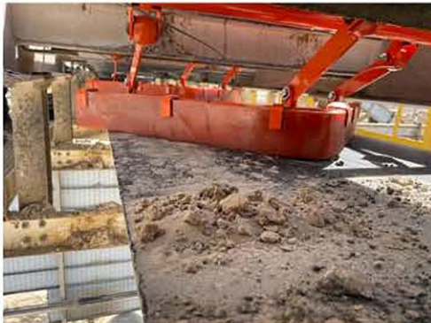
Figure 5. The V-plow diverts fugitive carryback to either side of the system, ensuring tail pulley health.
