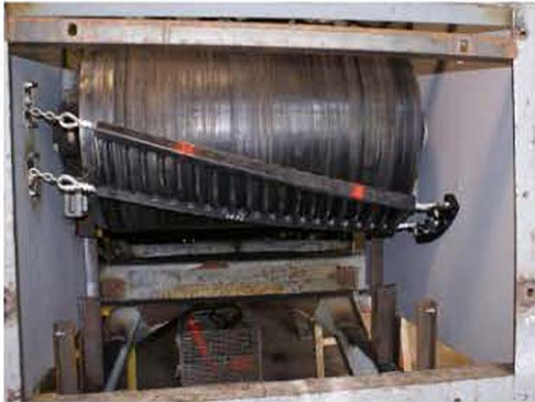
Figure 4. Innovative new cleaner designs require less monitoring and no tensioning.
