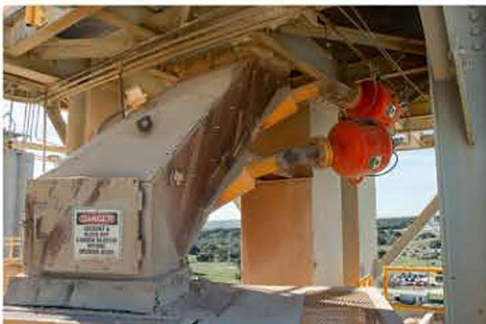
Figure 6. The direction of the cannon shot matches the stream trajectory to encourage constant flow.
