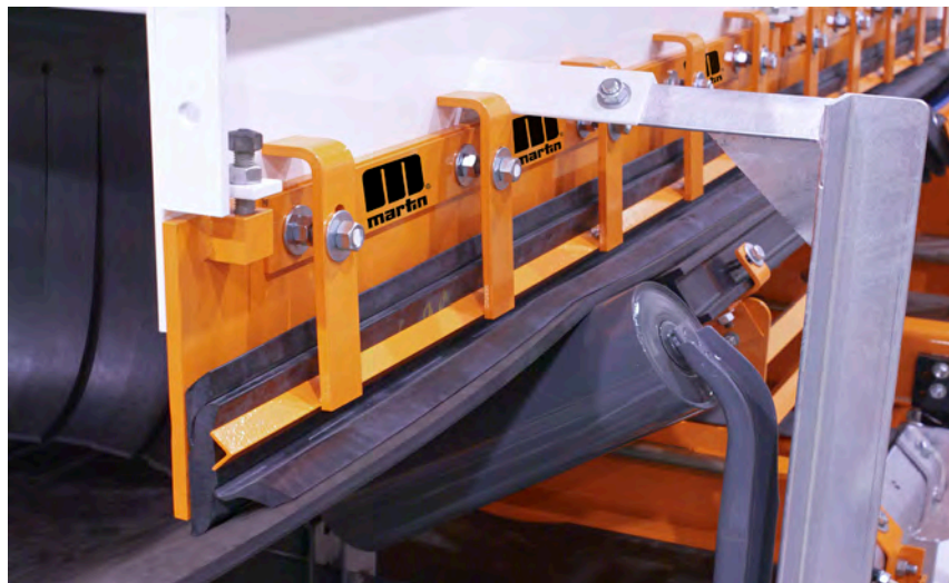
Figure 7. The raised skirtboard allows room for the external wearliner to perform its function and be changed easily from outside the system.
