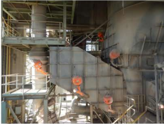
A series of air cannons can be programmed to deliver precisely-timed operation for maximum benefit.
