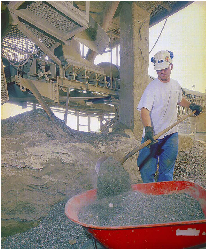
Figure 2. Fugitive material is an expense and potential hazard that can be prevented.
