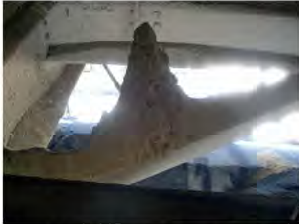
Figure 1. Carryback dislodged from the belt by a return idler.
