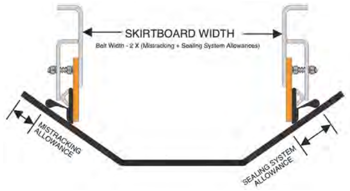
Figure 7. Mistracking allowance + sealing system allowance x 2 = skirtboard width.
