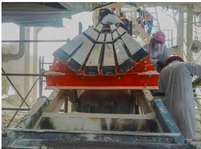
Figure 5. Cradles offer low friction surfaces at specified trough angles for superior belt sealing.
