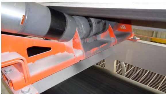
The load is carried by the generator's large support shaft, which is rigidly mounted to the idler support structure.
