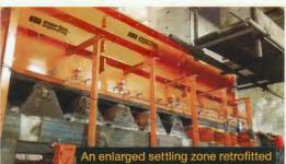
onto an existing conveyor enhances airflow control at a transfell point.
