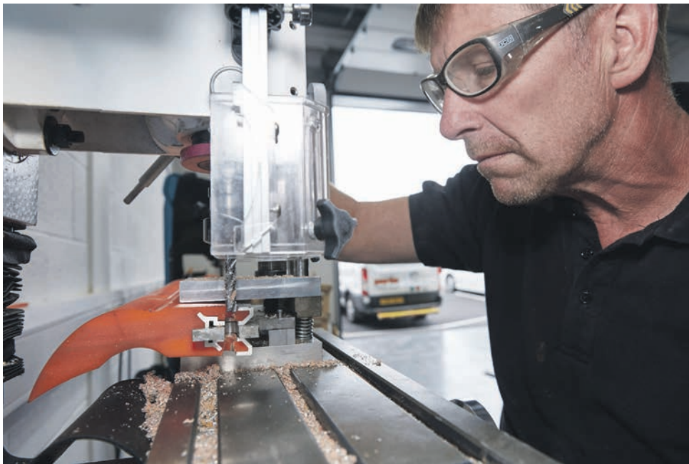
A technician mills a belt cleaner blade prior to installation.
