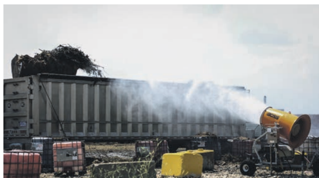
Gavlick's crew positioned the unit to cover the area where yard waste is loaded into trucks for transport to one of the company's composting facilities.
