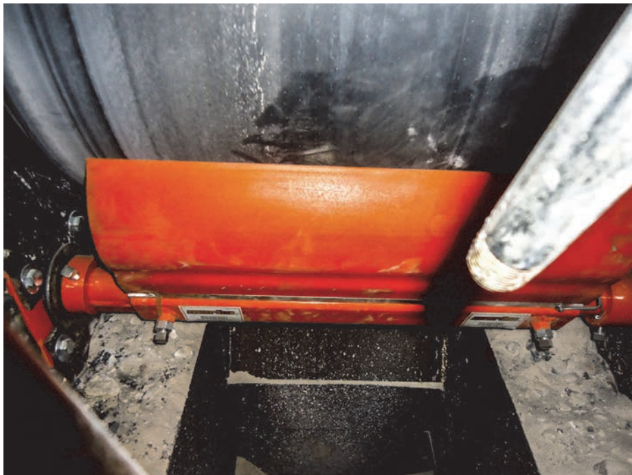
The Martin Engineering primary cleaner features a special polyurethane blend to deliver long service life.
