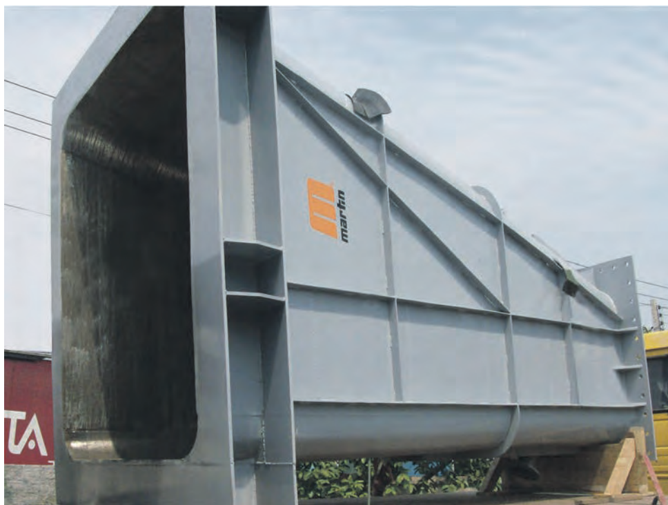
Arcoplate offers a solution to both excessive wear and material accumulation issues for chutes, hoppers, dump truck beds, excavator buckets, front loader shovels, and other bulk material equipment in need of protection.
