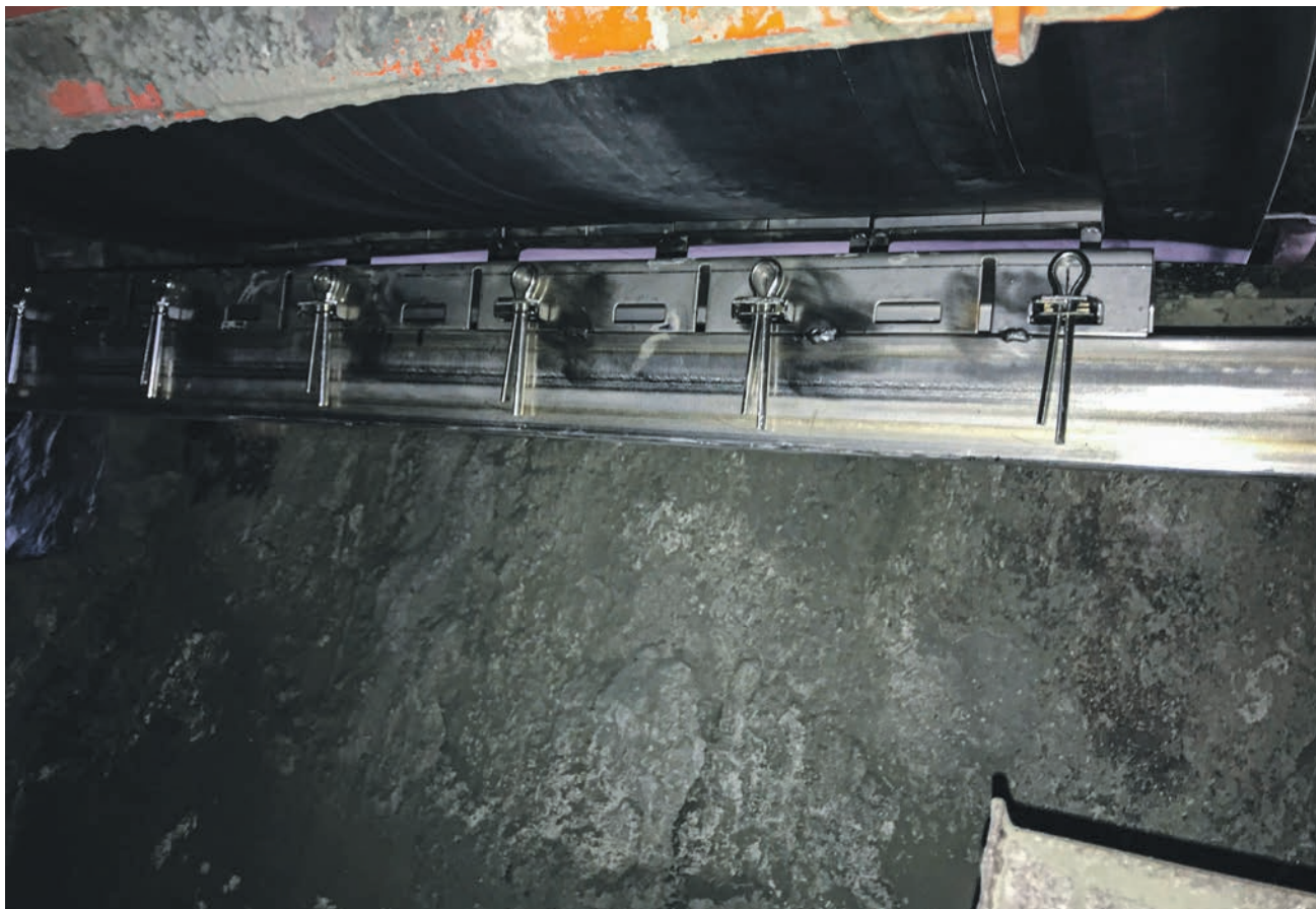
The unique stainless steel design incorporates a matrix of spring-loaded carbide tips.
