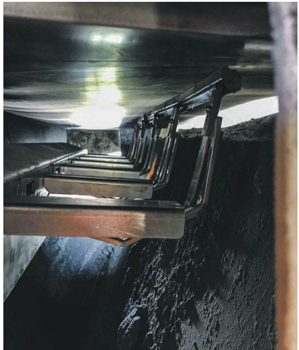
The new secondary belt cleaner is engineered to minimize maintenance and conveyor stoppages.
