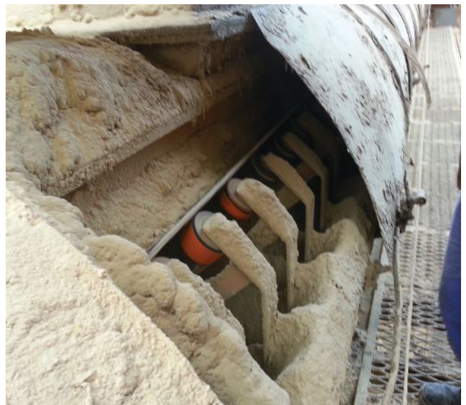
Dust and spillage clogs idlers, requiring them to be replaced and raising the cost of operation.
