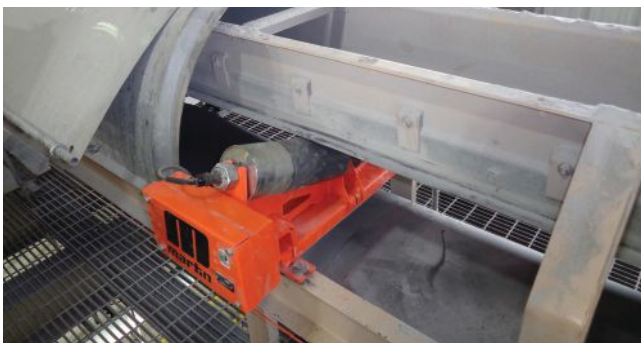
A single roll generator has enough power output to run a variety of accessories.
