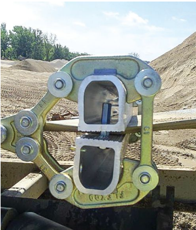
Belt clamps can be as small as two bars or as large as a giant vice.
