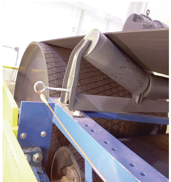
The pinch point between the belt and a carrying idler is one opportunity for an entrapment injury.
