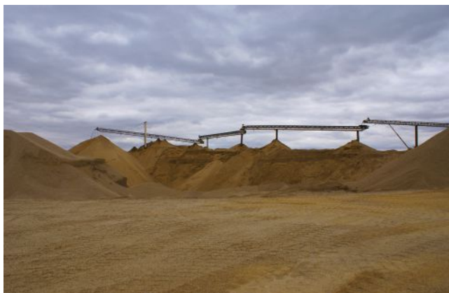
Inland sand is extracted and placed in stockpiles for transport to the processing plant.
