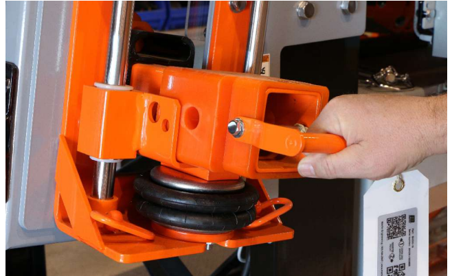
Figure 7: Ease of service should be a key element in any belt cleaner tensioning system.
