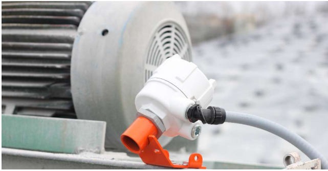
Figure 6: Sensors are used to back the blade away during stoppages or when running empty.
