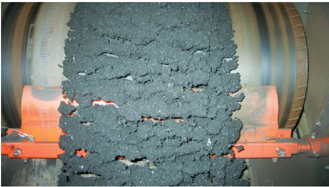
Figure 1: When the blade is wider than the material flow, its center may wear quicker than the outer edges.
